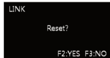
Factory reset is the function all setups of NRM-8000A are initialized.
