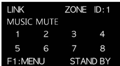
In case the point of contact is inputted with MUTE terminal at the back of NPX-8000, MUSIC MUTE phrase is displayed at the upper left. At this status, the device can be controlled, but the audio signal at NPX-8000 is not outputted.
